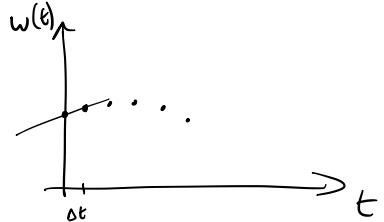
$$\left\{ \begin{array}{l} k(t+\Delta t) = k(t) + \underline{k'(t) \cdot \Delta t} \\ \omega(t+\Delta t) = \omega(t) + \underline{\omega'(t) \cdot \Delta t} \end{array} \right.$$
